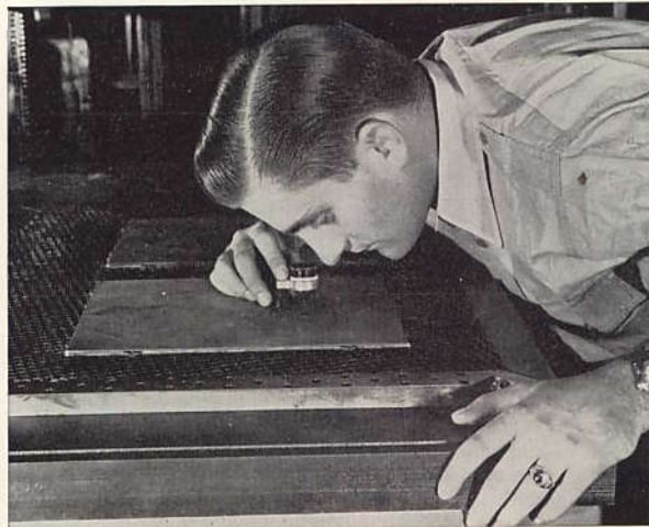
Check engravings for proper dot formation.
